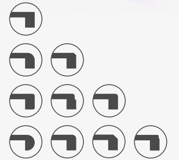
Examples of built-in edge profiles
