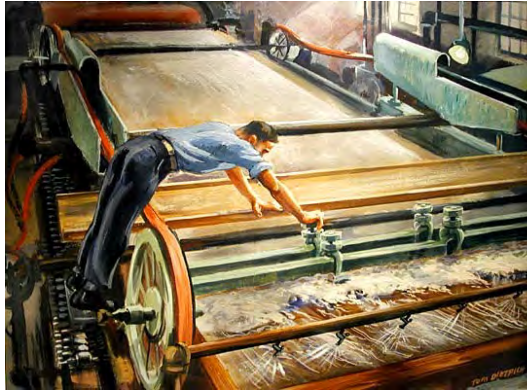
Old style headbox and forming table. A wood fiber/water slurry is metered onto a moving screen belt.
