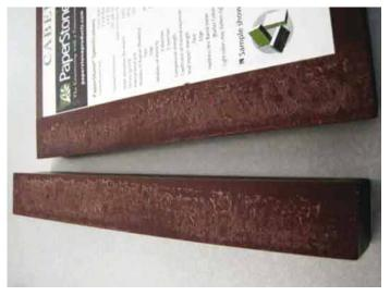
The surfaces were not sanded correctly before gluing, leading to weak cohesion and therefore a weak seam (see page 5).
