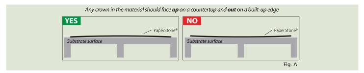
• Transfer drawing measurements to PaperStone panel and cut countertop pieces to size. *Allow enough overhang of material for built-up edge.*
