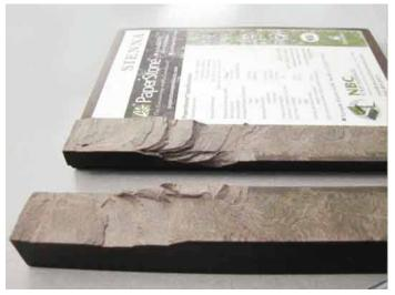
This photo shows how a correct edge seam leads to the panel breaking before being glued.
