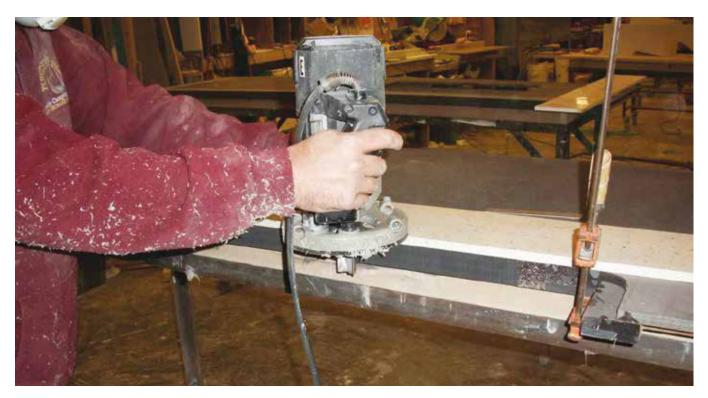
Step 1 Remove any excess adhesive and finish edges with a router and straight edge.
