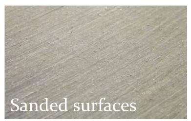
Using a sanding belt with 60/80 grit sandpaper, remove the layer of resin on the surface to be glued. Sand down to the level of the paper.
