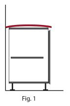
If the PaperStone panel is slightly curved, we recommend that the panel is placed with the "crown" facing up. (see Fig. 1)
