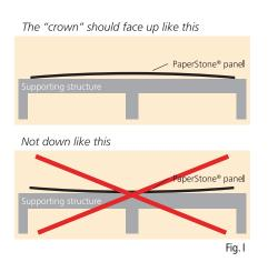
When the worktop is attached to the support frame of the cupboard, the crown will straighten and become level with the frame. In any case, the crown will not protrude more than 3,1 mm (on a total length of 75 cm).
